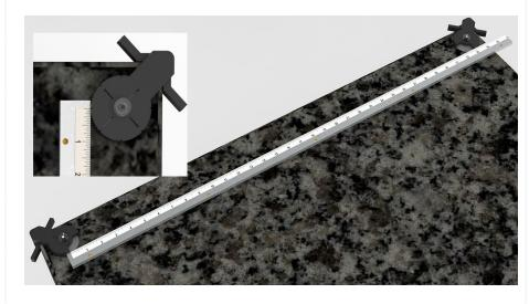
Note – we recommend that the extra length of the straight edge be no longer than 1/3 of the edge of the plate. This is to ensure that the straight edge does not move around when you are taking data. This can happen because as the straight edge gets longer relative to the plate edge, it tends to want to fall off the plate.
