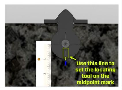
Position the straight edge with the *scale side* touching the Corner Locating Tool and position the zero point on the scale with the rotary edge on the locating tool.
