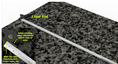
As before, place the A-703SP-LM fixture on the side recommended by Plane6 and place the target in the near position and hit Record. Continue taking data for the whole segment.
