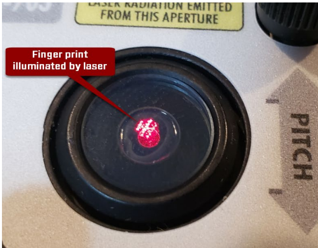
Figure 19 - Dirty vs. Clean Laser Window Example
