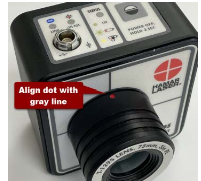
Figure 7 - T-1295/T-1296 Target with T-1295-AO-3 Lens installed correctly
