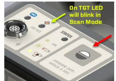
Figure 7 - T-1295/T-1296 Target with T-1295-AO-3 Lens installed correctly
