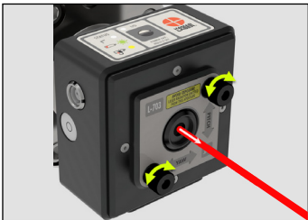
Step 5 - Turn on the T-1297 Target and go to Step 2, where it will connect to Plane6. Move the T-1297 to the far end of the straight edge and adjust the L-703SP's pitch/yaw angular knobs until the readout is within 5000 \mu\text{m} . (130 \mu\text{m} ).
