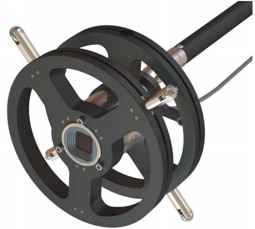
A-516-II 2-Axis Self-Centering Target
