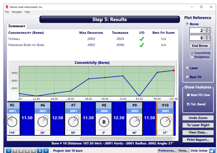
Bore9 – Step 5: Results – Concentricity Plot using Bore 2 & 8 as a reference.
