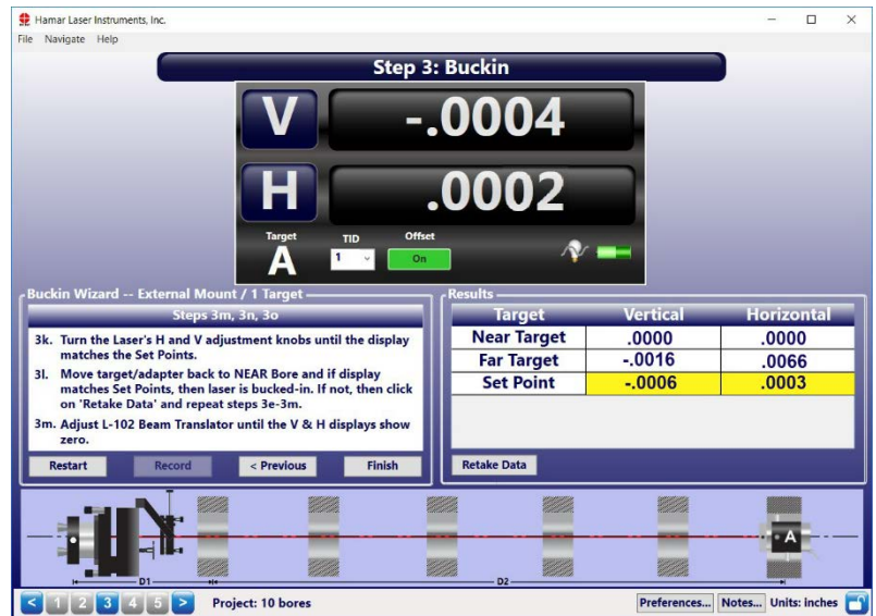
Bore9 - Step 3: Laser Steered to Zero (Bucked-In)
