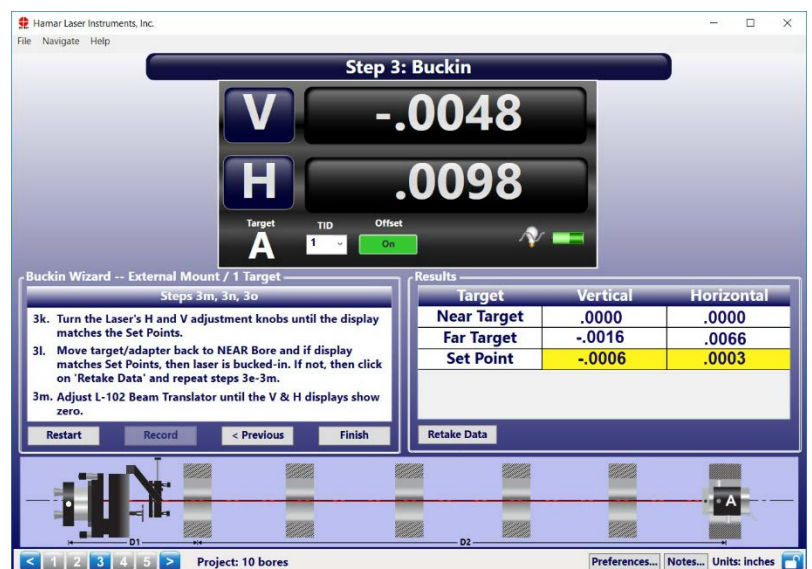
Bore9 - Step 3: Data Taken Far Bore and Set Points Calculated
