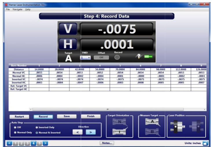
Bore9 – Step 4 – Data Recorded for All Bores
