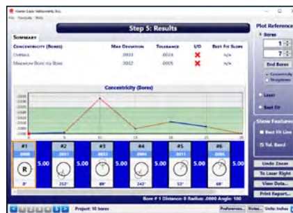
Bore9 Software showing plot of bore concentricity.
