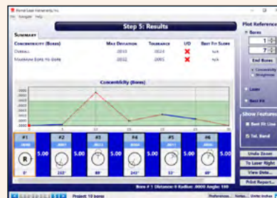
Bore9 Step 5: Results Concentricity Plot
