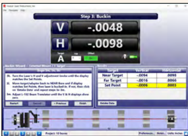
Bore9 Step 3: Buck-In with Set Points Calculated
