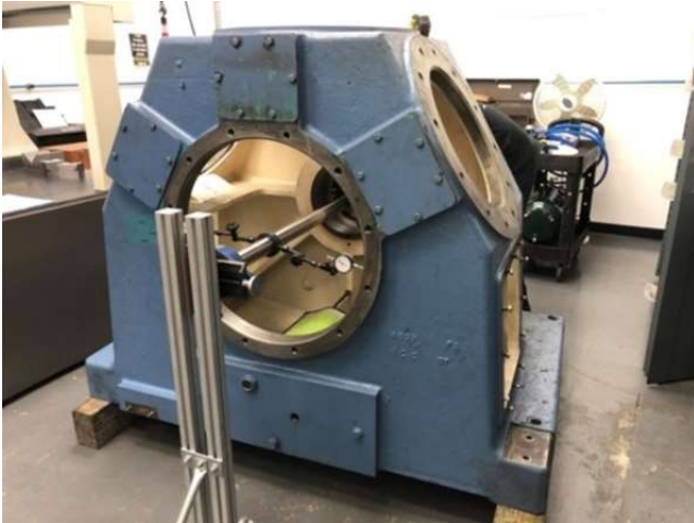
Hi-Tech's original dial indicator QC setup in compressor housing.
