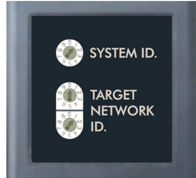
Figure 29 – Unitarget ID Switch set to 1
