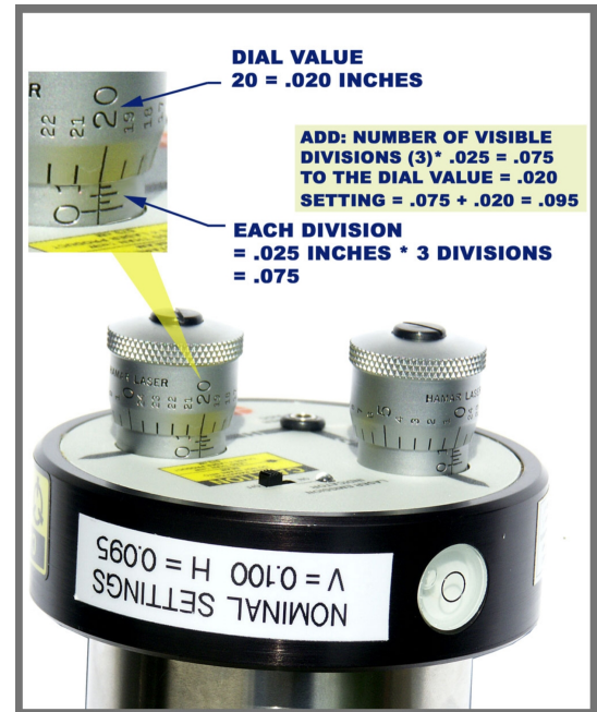
Figure 2 – Laser Micrometer Adjustments
