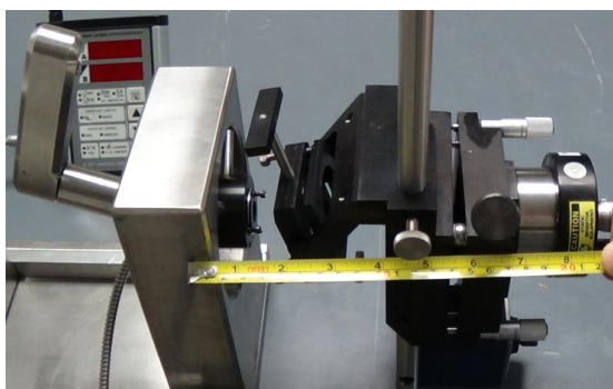
Figure 19-- D1 Distance Measurement: Center L-111 posts to mid-point of the target in Near Bore
