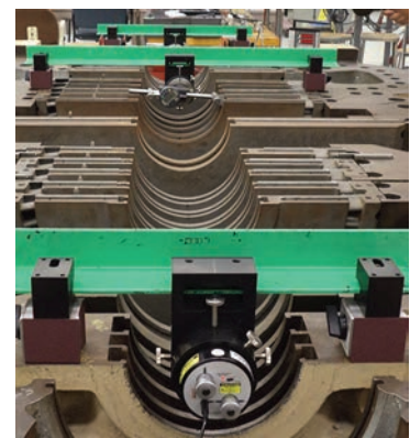
The L-706 Laser can be combined with our T-218T Turbine Target, half-bore fixtures and a bore sweep unit to make it the ideal system for aligning steam turbines
