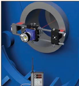
L-705/L-111 Laser and Stand Mounted on Bore Face
