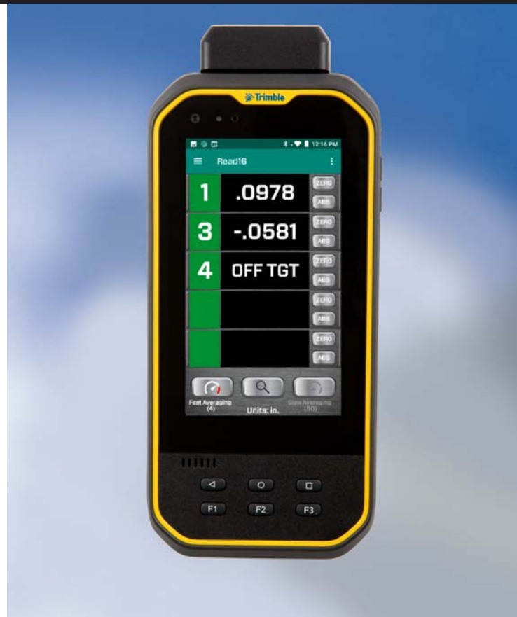
Read16 Android Software displayed on the R-1357-2.4ZB Wireless PDA Data Receiver
