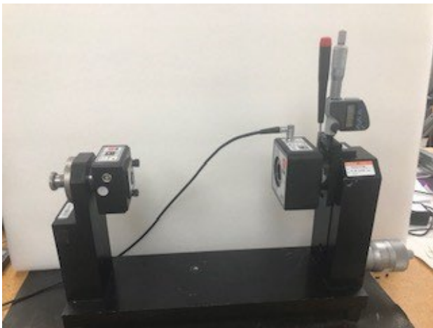
Figure 1 -- A-807 Calibration Fixture with X-Axis Translation and Angular Stage for T-212 and T-261 Targets and L-700/L-703/L-705/706 Laser Mount
