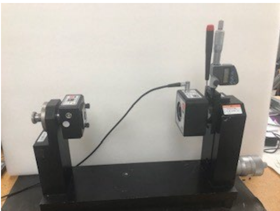
Figure 21 - A-807 Calibration Fixture with X-Axis Translation and Angular Stages and L-700/L-703/L-705/706 Laser Mount
