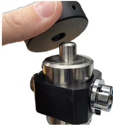
Assembling the A-808-212XY X-Y Stage Mounting Adapter with T-212 Target
