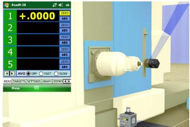
5. Rotate to 270 degrees. The reading is  $-.0023$ , which means the A rotation axis is tilting toward the X-Axis by  $.0023$  in 18 inches.
