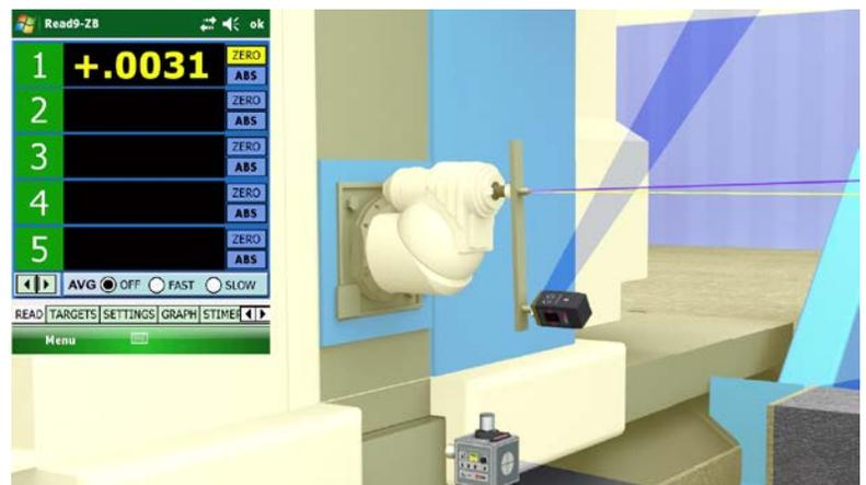
3. To compare to the X-Axis, start at 90 degrees and zero the PDA. Rotate to 270 degrees. The -.0019 reading indicates that the spindle axis is pointing to the left relative to the X-Axis.
