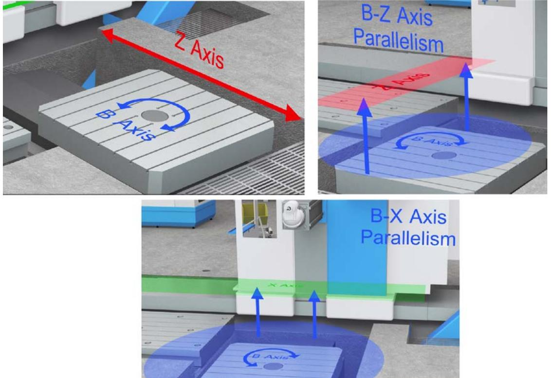
1. To check the B rotation, move the target to one of the corners of the table. Zero the display and then rotate the table 90 degrees.
