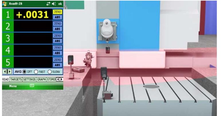
5. Plane5 analyzed the data and found that the flatness of rotation is **.0010" TIR** and the parallelism to X is **.0011 in./ft.** and **.0002 in./ft.** to Z.
