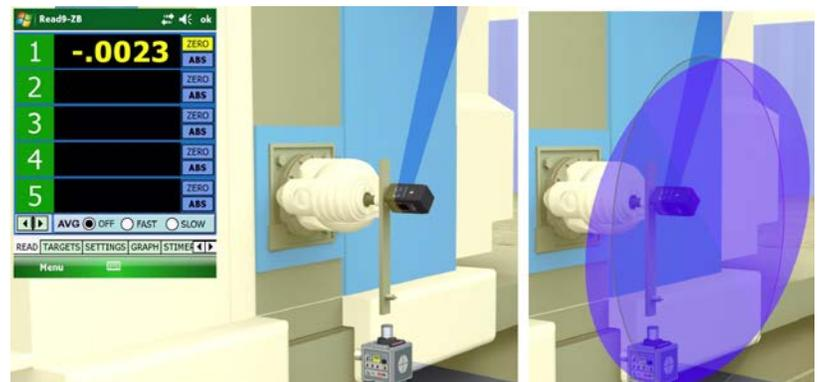
6. The last A-Axis check is to measure the flatness of the rotation. Take measurements every 45 or 90 degrees and use Plane5 to calculate the flatness.
