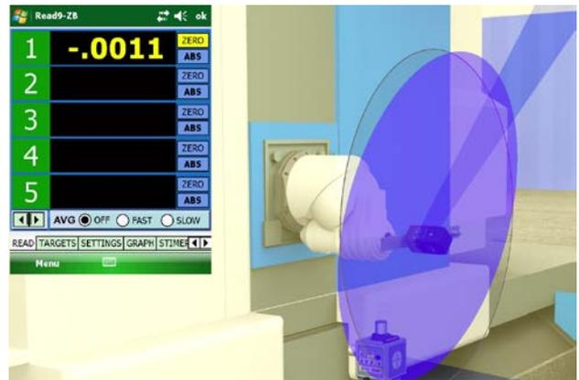
4. Rotate to 90 degrees and again, zero the target.
