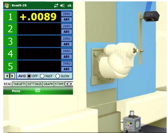
2. As with the A-Axis, begin at 0 degrees, zero and rotate 180 degrees. The .0031 reading indicates the spindle axis is pointed upward relative to the Y-Axis.
