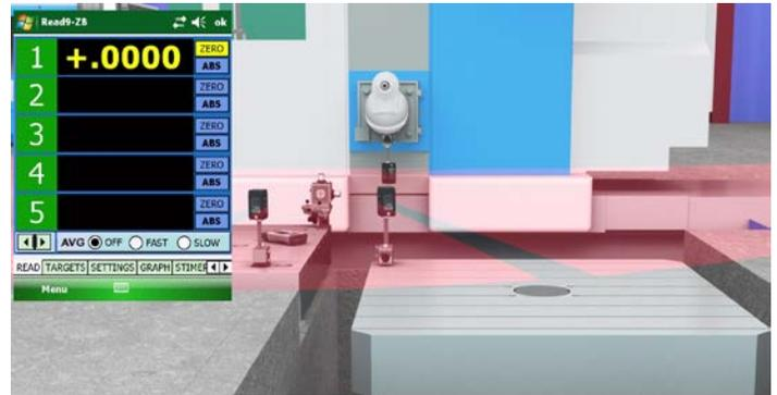
2. The display shows  $+.0024$ , indicating that the table rose by  $.0024$  as it rotated. Therefore, the rotation plane is sloping up from left to right relative to the main table (recall that the main table was the reference for the horizontal red laser plane).
