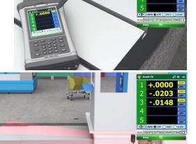
6. Looking at the data for Targets #1 and #2, adjust the Pitch-Axis knobs on the laser until the two values are equal. Switch to Targets #1 and #3 and adjust the Roll-Axis knobs on the laser until those two values are equal. Now the target values for all three targets are equal and the laser plane is aligned to the table.
