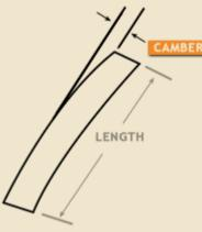
side edge from a straight line, the straightness of the edge of sheet or slitting operation. Camber is the departure of a side edge of sheet or Extreme camber contributes to curve, finished part.
