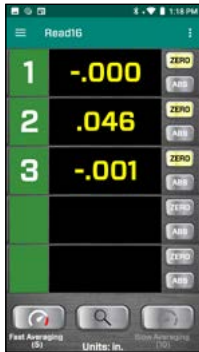
R-1358-2.4XB PDA Readout with laser aligned to reference targets, showing a roll measurement
