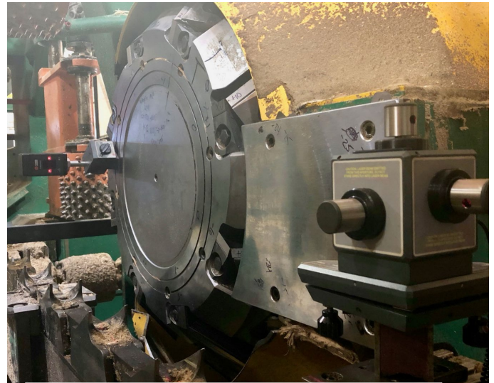
L-743 & A-1519-2.4ZB Measuring Blade Parallelism
