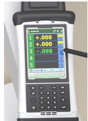
R-1356-2.4ZB PDA Readout showing values for Targets #1, 2 & 3
