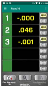
R-1358-2.4XBE PDA Readout with laser aligned to reference targets, showing a roll measurement
