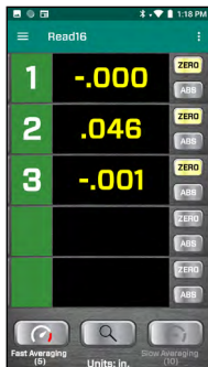
R-1357-2.4XBE PDA Readout with laser aligned to reference targets, showing a roll measurement
