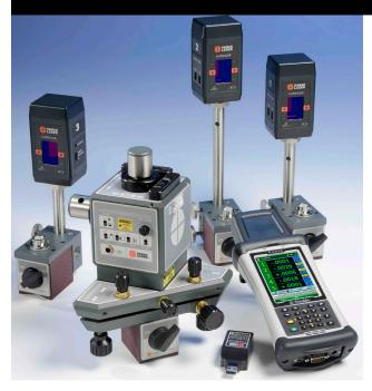
The L-732 Precision Dual Scan® Laser is the ideal instrument to quickly and accurately calibrate the geometric alignment of almost any kind of injection molding machine. It is a powerful tool that not only finds, but also fixes geometry problems, all in a fraction of the time needed with conventional methods.
