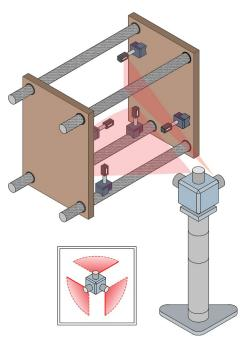
Aligning an Injection Molding Machine
