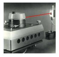
The Model L-711 laser alignment system was the first such system to feature a pentaprism that created a manually sweeping precision laser plane. The groundbreaking alignment device was accurate to less than 0.5 arc-sec (0.0025 mm/m)!
