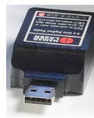
A-910-2.4XBE Computer Interface 2.4GZ wireless data receiver for laptops to display data in Plane5 or other HLI program.
