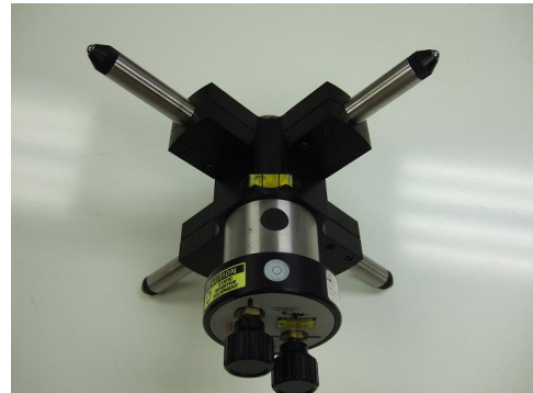
Figure 13 – Laser mounted in bore adapter
