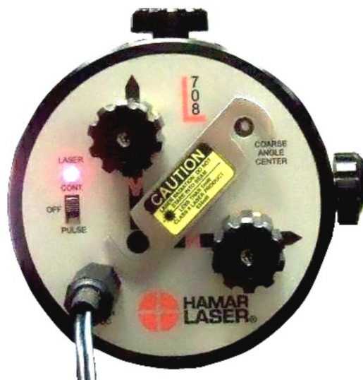
Figure 3 – Fine Adjust Tool Indicator in the OUT position
