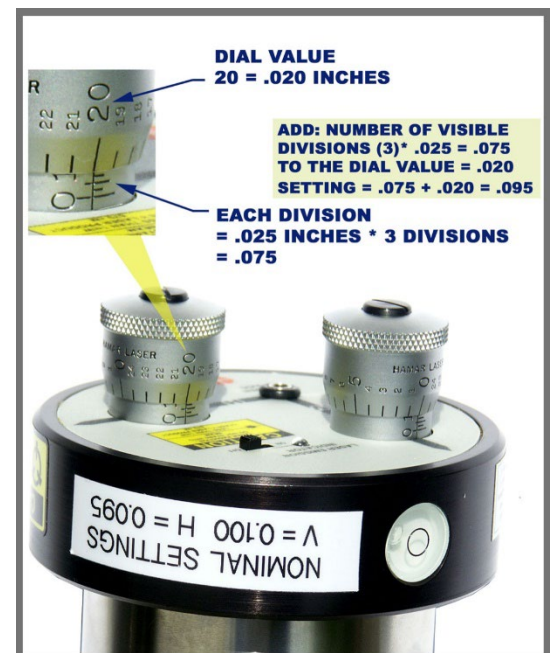
Figure 2 - Adjusting L-706 Micrometers
