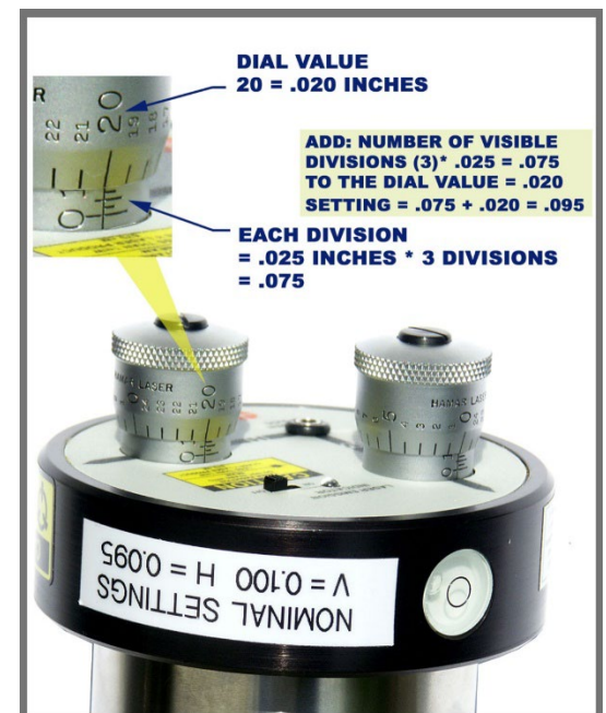
Figure 2 - Adjusting L-706 Micrometers
