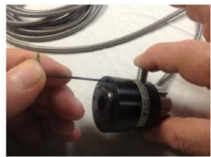
Figure 11 – Insert leg and tighten set screw in the A-510STA to push the leg against the OD of the A-510 Target
