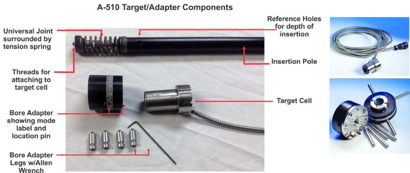
Figure 9 – A-510 Target/Adapter Components (left) and A-510 Target with Adapters (right)
