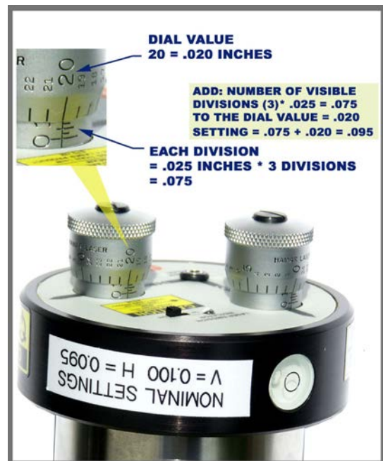
Figure 2 – L-705 Laser Micrometer Adjustments
