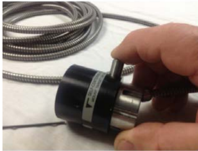
Figure 11 – Insert leg and tighten set screw in the A-510STA to push the leg against the OD of the A-510 Target
