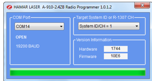
Figure 34 – A-910 Utility showing the COM Port, System ID and Channel settings
