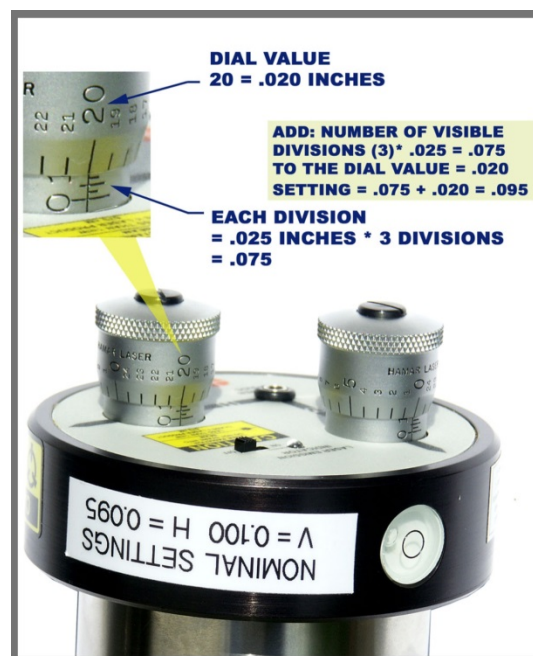
Figure 2 – Laser Micrometer Adjustments
