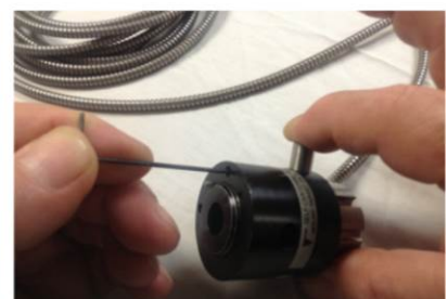
Figure 31 – Insert leg and tighten set screw in the A-510STA to push the leg against the OD of the A-510 Target
