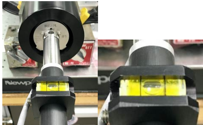
Figure 29 -Insertion Pole Level Assembly with bubble leveled.
