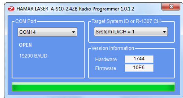
Figure 49 – A-910 Utility showing the COM Port, System ID and Channel settings
