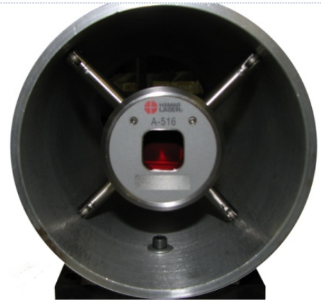
Figure 28 - Self-Centering Adapter Inserted into a Bore at 45 Degree Angles Relative to 12:00
