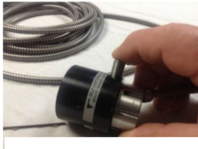
Figure 31 – Insert leg and tighten set screw in the A-510STA to push the leg against the OD of the A-510 Target
