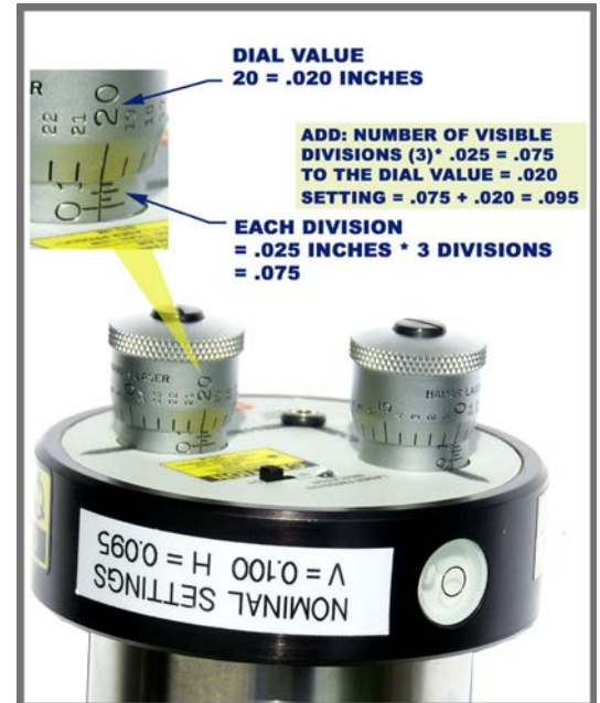
Figure 19 - L-705 Laser Micrometer Adjustments
