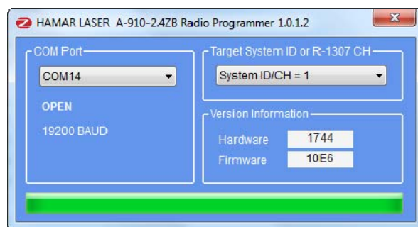
Figure 29 – A-910 Utility showing the COM Port, System ID and Channel settings
