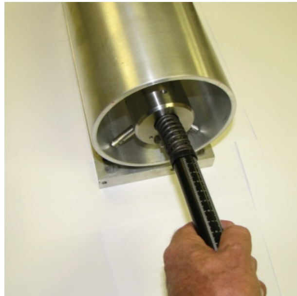
Figure 5 – Inserting the A-516 Target into the bore
