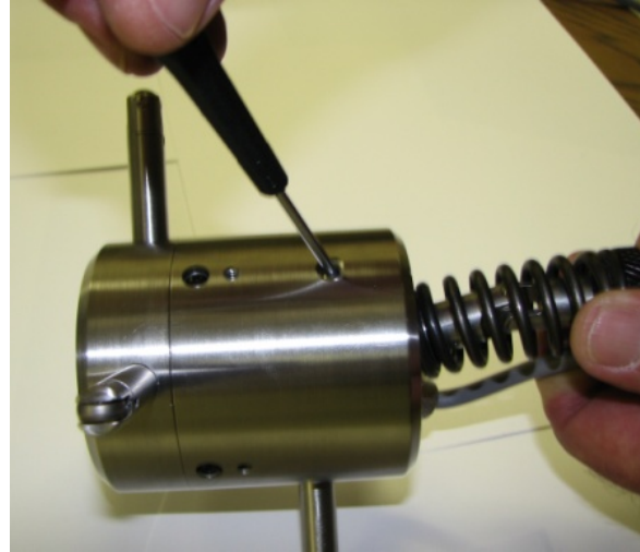
Figure 3 – Attaching the A-516P Pole Assembly
