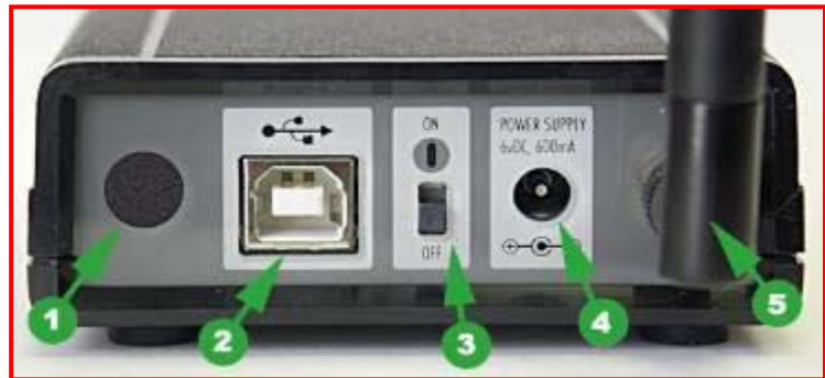
Figure 25 – The A-910 Radio Transceiver/Hub REAR PANEL
