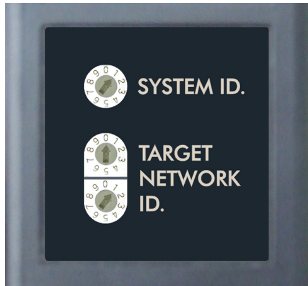
Figure 32 – Unitarget ID Switch set to 1
