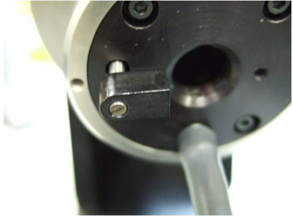
Figure 5 – T-218 Flip Lever seated in proper position
