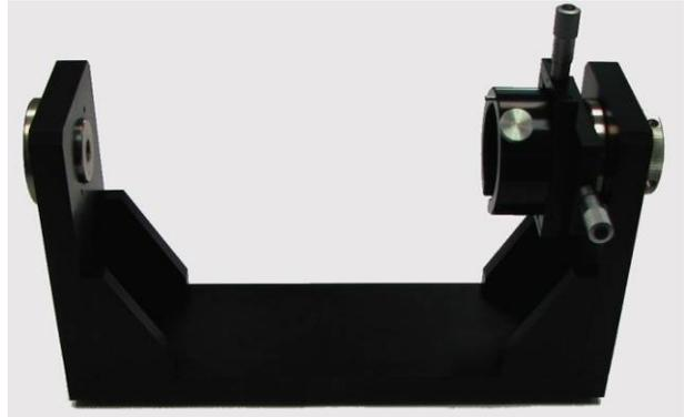
Figure 1 -- A-808 Calibration Fixture with X-Y Target Stage for T-218/219 Targets and L-705/706 Laser Mount
