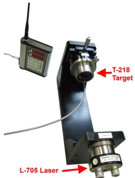
Figure 2 – Laser and Target mounted in A-808 fixture
