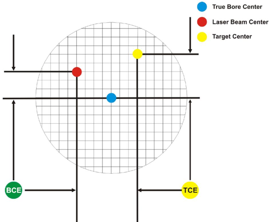
Figure 81 – Three centers of bore alignment
