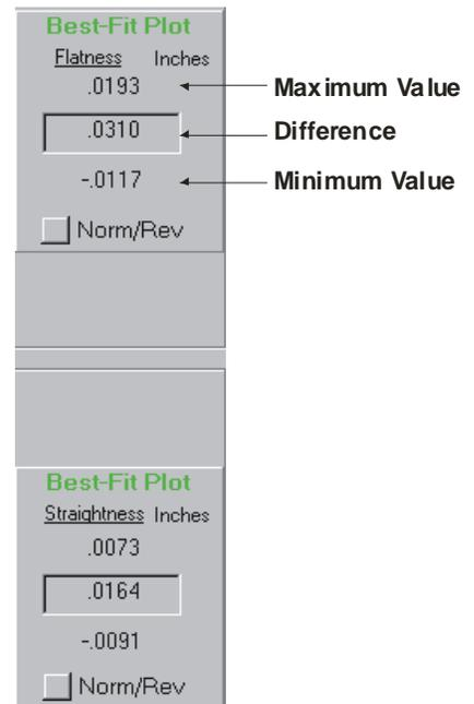
Figure 75 – Maximum, Difference and Minimum Values for Best Fit Plot
