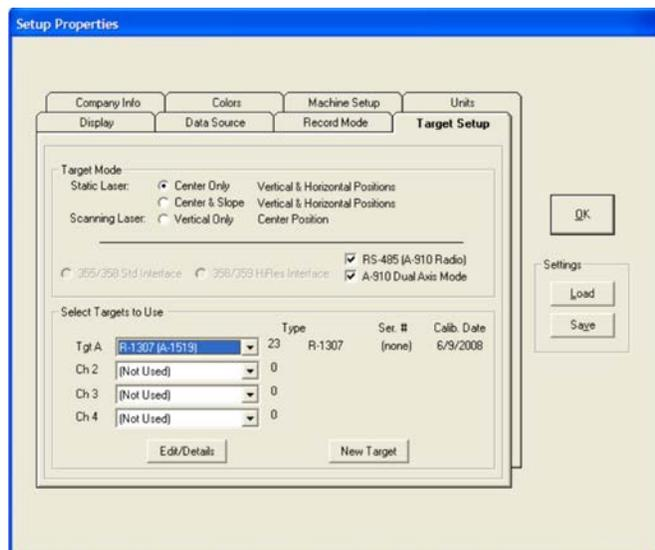
Figure 21 – Selecting the A-1519 Target with the R-1307 Readout
