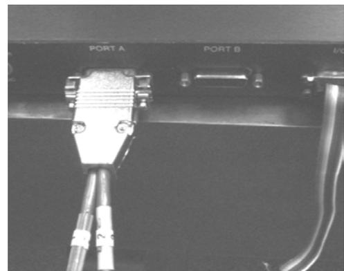
**Figure 1** – T-237C Target Adapter Cable Connected to Port A of the R-355 Interface
