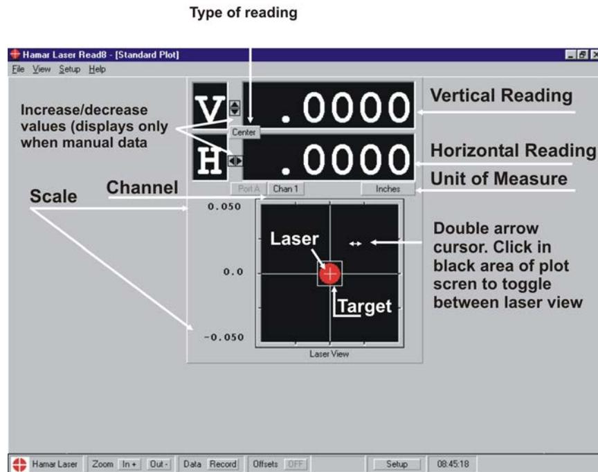
Figure 29 – Standard Plot Screen (One Target Showing Center Only)
