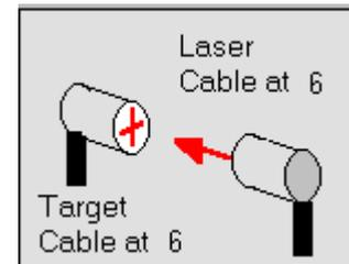
**Figure 52 –** *Align Laser Offset – Second Reading – (laser and target in normal position).*
