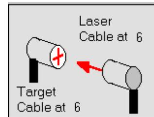
**Figure 54 –** *Align Target Offset – Second Reading – (laser and target in normal position).*
