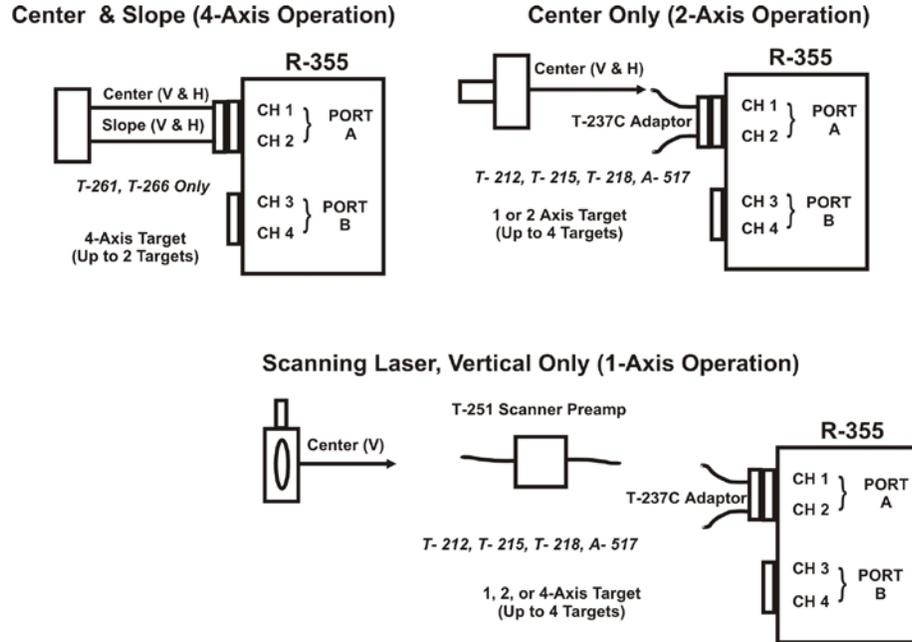
Figure 2 – Connecting to the R-355 Computer Interface
