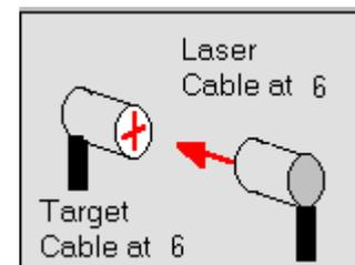
**Figure 49 – Spindle Offset – Third Reading (laser and target in normal position)**
