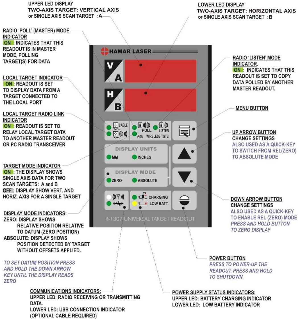
Figure 6 -- R-1307 Readout Control Panel Features
