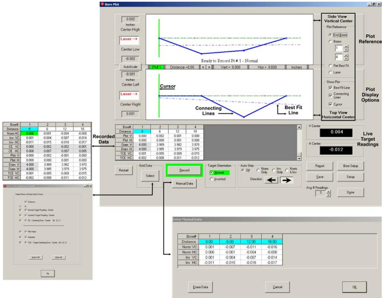
Figure 41 – Bore Plot Screen showing Manual Data Screen and Grid Selection
