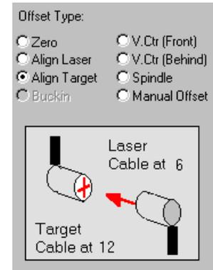
**Figure 53-** *Align Target Offset – First Reading (target inverted)*
