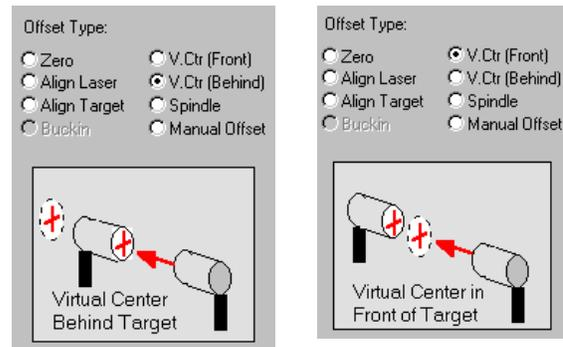
Figure 61 – Setup for Virtual Offsets
