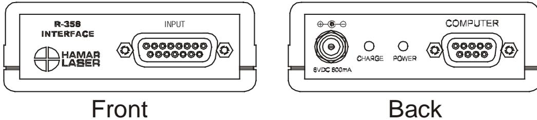
Figure 4 – R-358 Interface Connections
