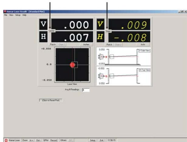
Figure 32 – Center and Slope Buttons
