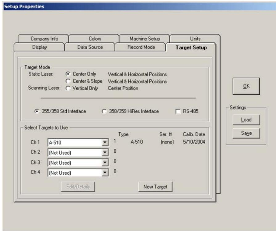
Figure 7 – Setup Menu showing Target Setup
