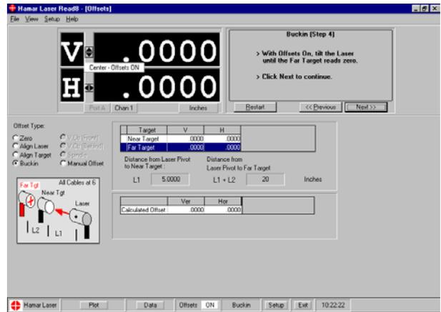
Figure 59 - Buckin Offset Screen – Zero and Remove Offsets (Step 4)
