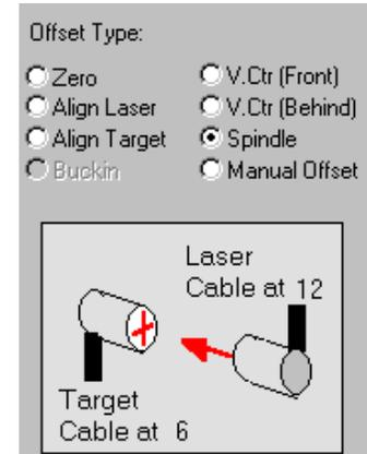
**Figure 47 – Spindle Offset – First Reading (laser inverted)**
