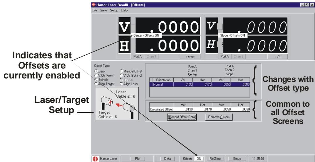
Figure 44 – Offsets Screen Showing Zero Offsets Display
