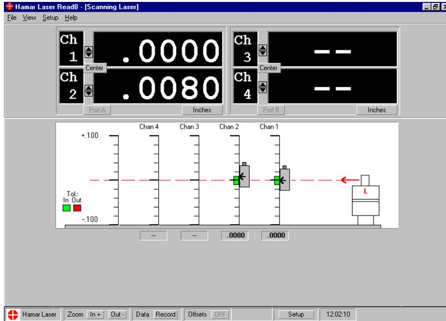
Figure 39 – Scan Plot showing two targets connected to Channel 1 and Channel 2
