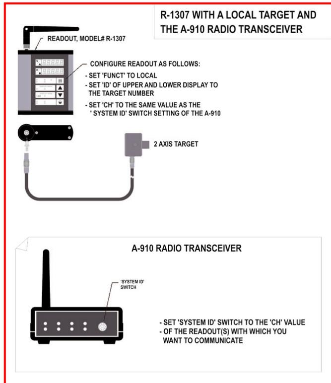
Figure 93— R-1307 with Cabled (Local) Target and A-910 Radio Transceiver
