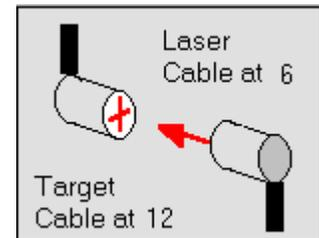
**Figure 48 – Spindle Offset – Second Reading (target inverted)**
