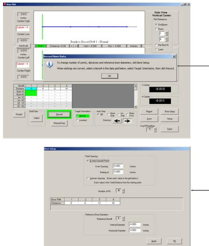
Figure 40 – Initial Bore Plot screen with Bore Setup
