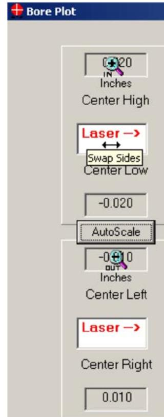
**Figure 42** – Changing laser orientation and using the AutoScale and Zoom features
