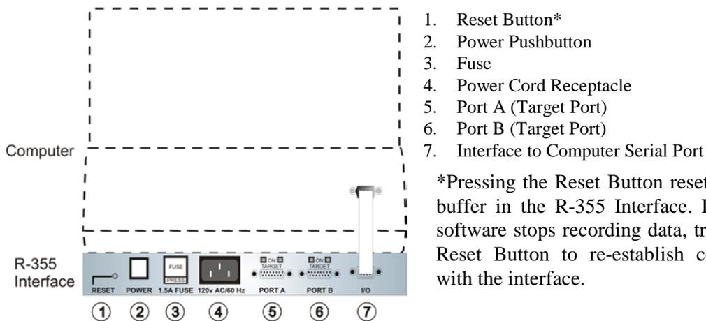
Figure 3 - R-355 Computer Interface, Rear View
