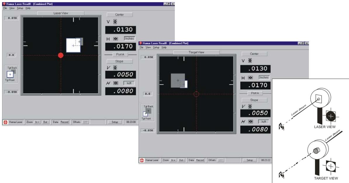
Figure 37- Combined Plot Screen, 4-Axis Target Showing Center and Slope readings, Laser View and Target View
