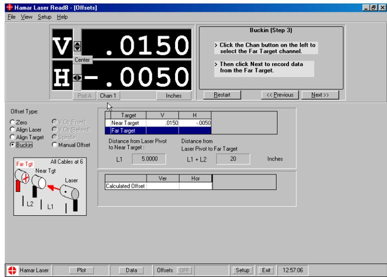
Figure 58 – Buckin Offset Screen – Recording Far Target (Step 3)
