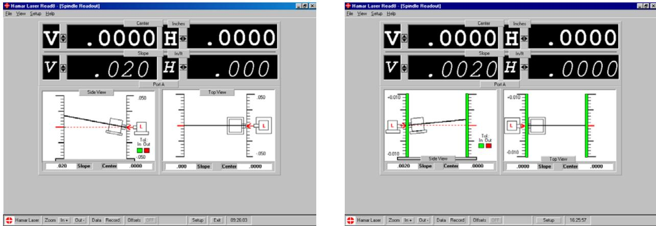
Figure 38 - Spindle Plot Screen, 4-Axis Target Showing Center and Slope readings and alignment setup side change
