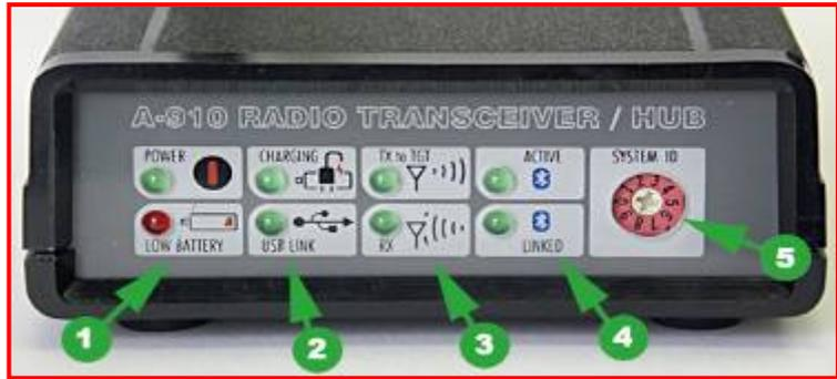
Figure 84 – The A-910 Radio Transceiver/Hub FRONT PANEL
