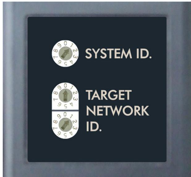
**Figure 92** – Unitarget ID Switch set to 1
