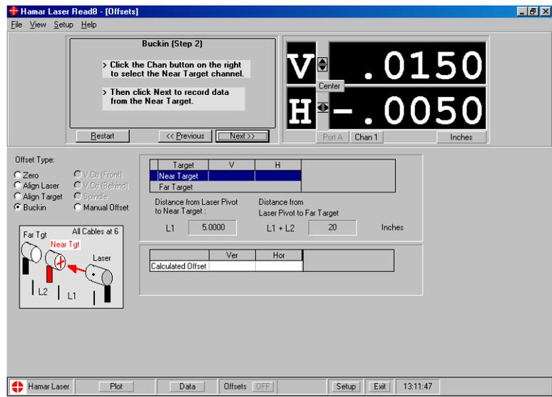
Figure 57 – Buckin Offset Screen – Record Near Target (Step 2)
