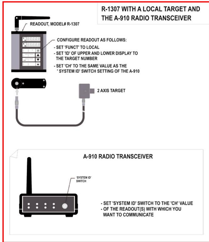
Figure 86 -- R-1307 with Local Target and A-910 Radio Transceiver
