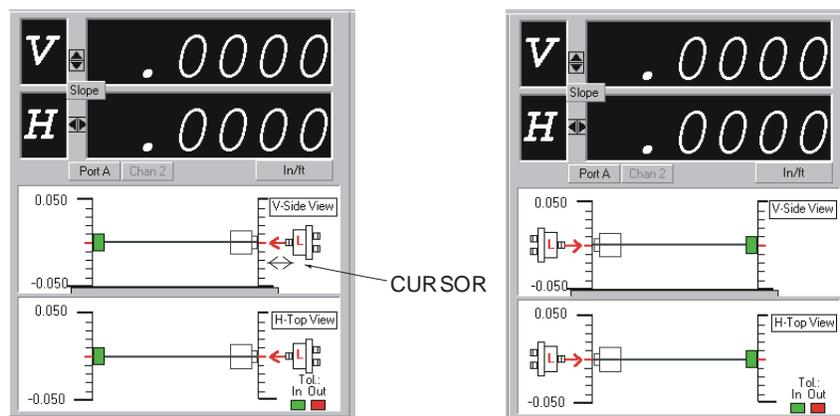
Figure 36 – Changing the Alignment Setup Perspective in the Slope Display
