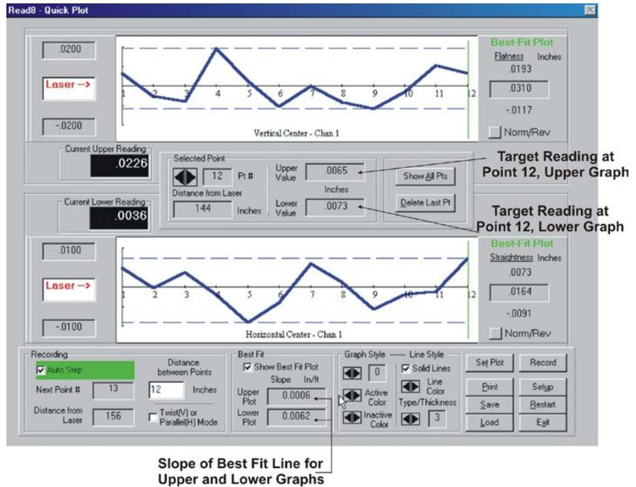
Figure 74 – Target readings by point and slope of Best Fit line.
