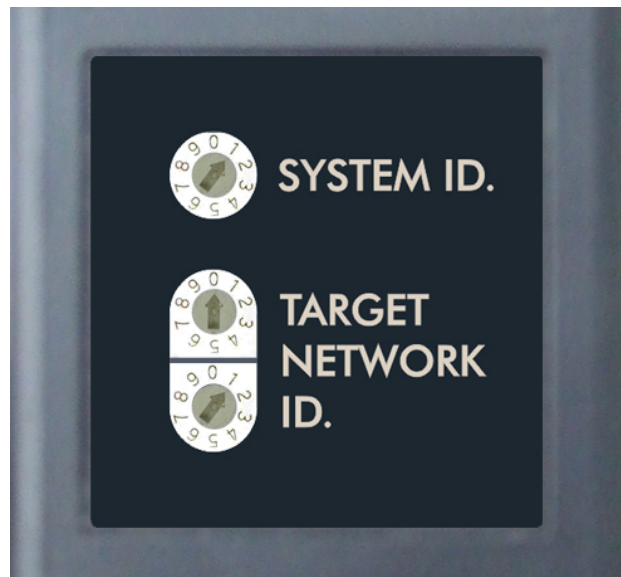
Figure 16 – System ID Switch set to 1
