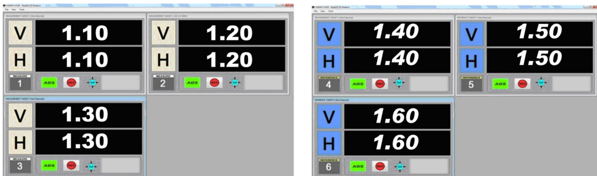
Figure 16 – Results of the View Menu, showing Measuring Target Readings (left) and Reference Target Readings (right)
