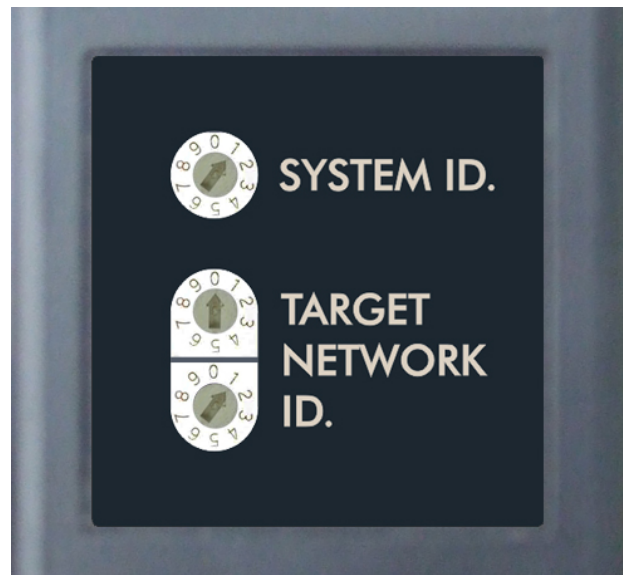
Figure 28 – Unitarget ID Switch set to 1
