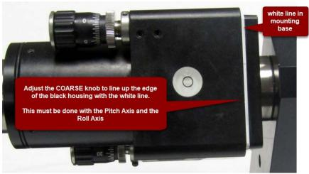
Figure 11—Returning the L-702 Pitch/Roll Adjustments to the middle of their range
