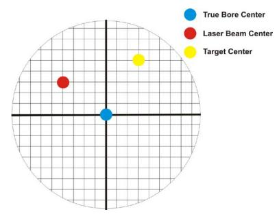
Figure 19 – Target in the NORMal position
