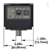
Figure 8—L-702 Mounting Stud
