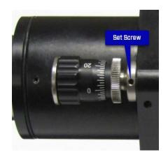
Figure 4– Differential Micrometer
