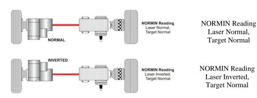
Figure 21—Taking NORMIN Readings
