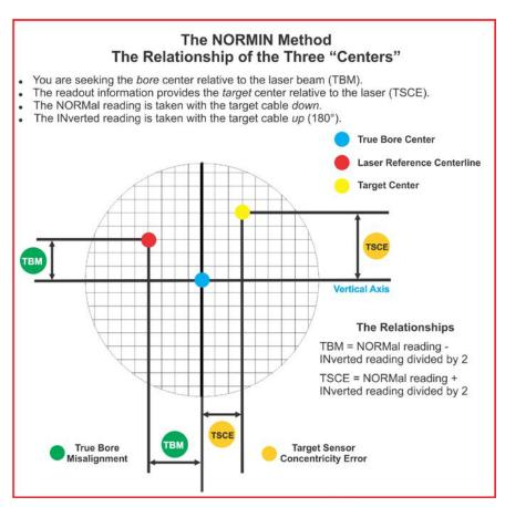
Figure 18 -- Three centers of bore alignment
