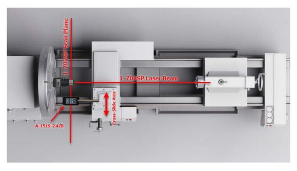
To measure a cross-slide or a machining axis of a multi-turn machine, the A-1519-2.4ZB Single-Axis Wireless target is needed to measure the scanning plane. The data values can be sent to our: R-1356-2.4ZB PDA Readout, R-1308 Single-Axis Readout or the R-1307W-2.4ZB 2-Axis Readout.
