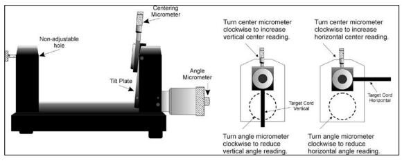
Figure 22—Model A-807 Calibration Mounting Fixture
