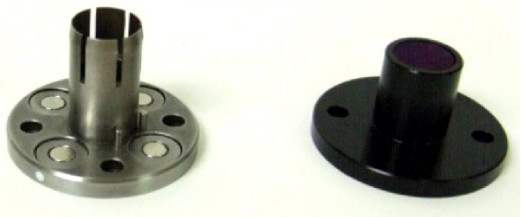
Typical target adapter and optional target light shield for the T-219 Target
