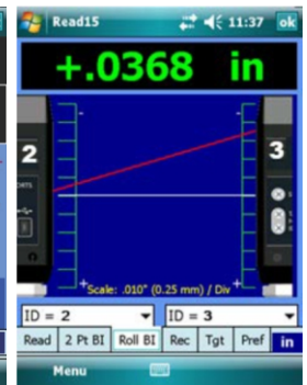
Roll Buck-In Tab showing the alignment of the laser to Targets 2 and 3.
