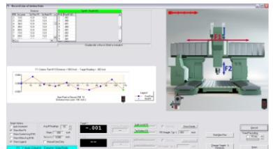
The **RECORD LINE OF MOTION DATA** screen displays live target data and the straightness tolerance for the selected line of motion in graph format. The graph is updated *as the data is recorded*. After each point is recorded, the cursor automatically moves to the next point and the least-squares, best-fit line is calculated. Multiple measurement “runs” and bi-directional data can also be recorded for each line of motion.
