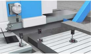
2. For straightness, mount Target #2's post into the side hole in the magnetic base to pick up the green laser plane. Adjust the pole length for Target #2, turn on the green laser and zero the display.
