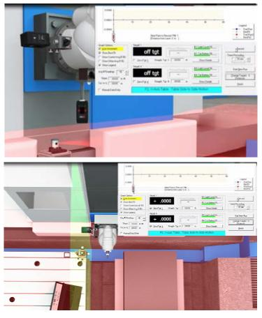
3. The red plane measures the flatness of W, W-Y squareness and parallelism to Z (in Y). The software records the straightness of W and calculates the squareness and parallelism to the other axes. The results show .0003" for straightness and .0011" for flatness.
