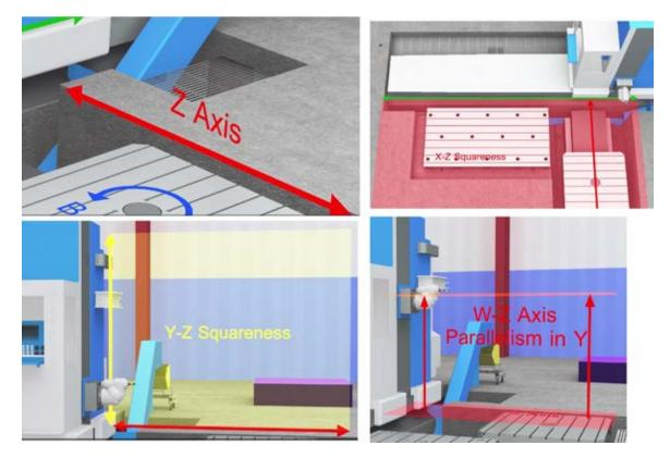
1. Leave the laser in position and re-position the targets. To measure Z-Axis flatness, use the red laser plane with Target #1 on the table.
