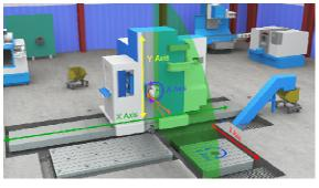
1. To measure the Y-Axis, move the second target to the side of the spindle and adjust the column and target height to center the laser in the window.
