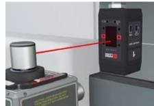
2. Turn on the rotation for both laser planes. The Gold Laser (top left) measures X-Axis Straightness and the Red Laser (bottom left) measures Flatness.
