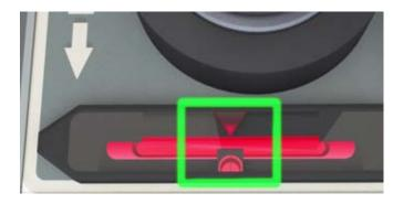
3. Place Target #1 at a location next to the laser and mark the outline of the magnetic base for good repeatability. Point the laser at the target window and adjust the target height until the laser beam is centered.
