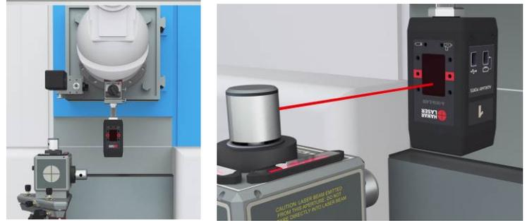
2. Turn on the rotation for both laser planes. The Gold Laser (top left) measures X-Axis Straightness and the Red Laser (bottom left) measures Flatness.
