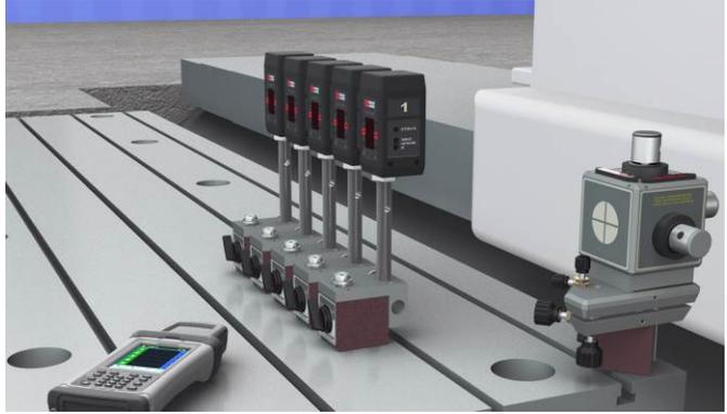
2. Level the Pitch-Axis level via by using the coarse and fine adjustments to line up the edges of the bubble. Repeat the process with the Roll-Axis level vial. Now the red laser plane is level to earth
