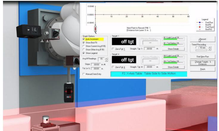
2. Zero Targets #1 and #4. The green plane measures the straightness of W, W-X squareness and parallelism to Z (in X).
