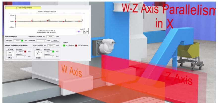
6. For Z squareness to X and Y, the Machine Tool Geometry program subtracts the Best-Fit slope of Z from the Best-Fit slopes of Y and X and calculates the squareness. Therefore, the result for the squareness of Z to X is .0002 in/ft, which means the Z-Axis is tilting to the left.
