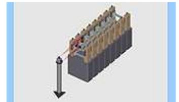
The L-742 can also be used to check the squareness of the support wall to the machine bed by taking advantage of the L-742's built-in squareness.
