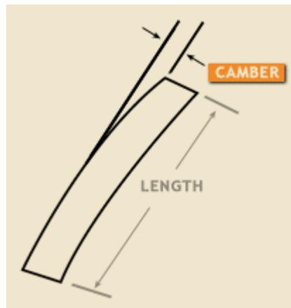
side edge from a straight line, the straightness of the edge of sheet or slitting operation. Camber is the departure of a side edge of sheet or Extreme camber contributes to curve, finished part.
