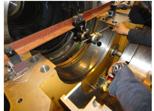
A-502 Turbine Fixture with A-501 Bore Sweep Unit
