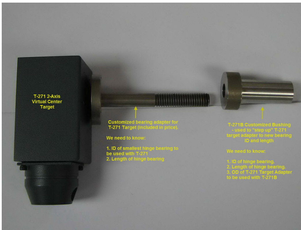
L-271 2-Axis Virtual Center Target with Customized Bearing Adapter and T-271B Customized Bushing with criteria for customization
