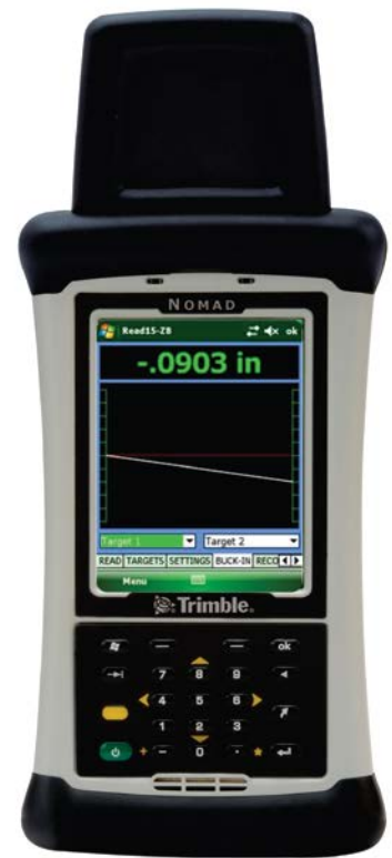
Read9 ALIGN Screen showing the difference between Target 1 and Target 2 relative to the laser plane.
