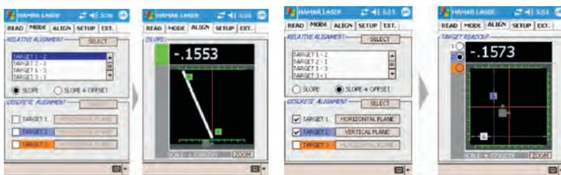
The ALIGN screen is a graphic representation of the target readings, showing alignment as defined in the MODE screen. The graphic display scales up automatically to fit the readings, and it can be downscaled by clicking the ZOOM button in the bottom right-hand corner. Screens for both Relative (left) and Discrete (right) alignment modes are shown.
