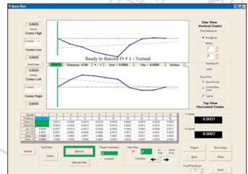
Bore8 Software showing plot of bore straightness.
