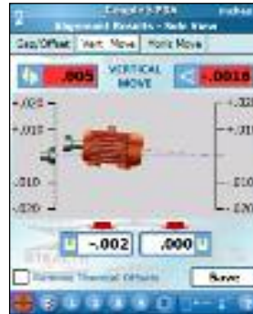
Move Screen – Live in both offset and angular axes, the Move Screen instantaneously shows the movement of the motor during alignment making it easy to align the motor.
