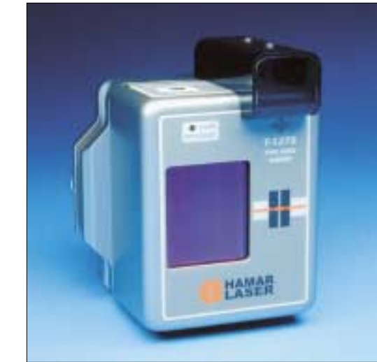
Target The T-1275 features a true 5-axis target that reads both horizontal and vertical center and angle measurements simultaneously. Target data is sent instantly via an IR link to the CPU for real-time processing, analysis and display of misalignment data. Largest cell size on the market accommodates thermal growth offsets up to 1".
