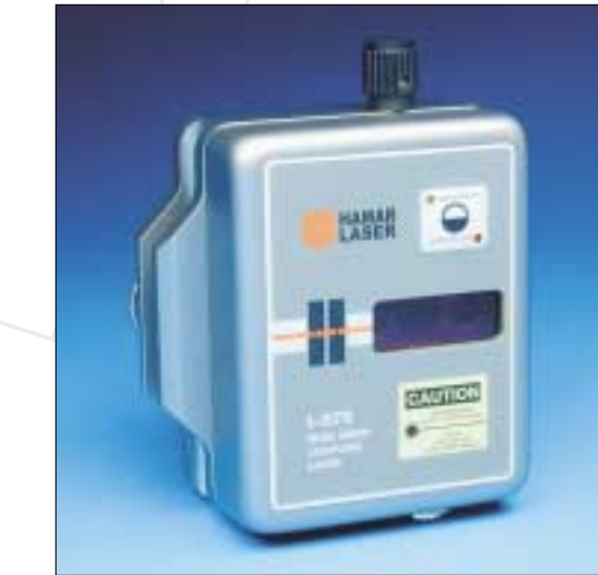
Laser The L-575 uses two adjustable, visible-diode Class II laser beams with an operating range of up to 30'. Angular accuracy of the system is guaranteed to 10 micro radians. Set-up time is minimal. In most cases, you can show misalignment data and calculate shims and moves in as little as 5 minutes.
