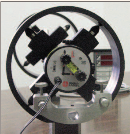
Using the A-514 Self-Centering Target Adapters, the L-708 can be mounted in the first reference bore and centered to .0006" (0.015 mm).
